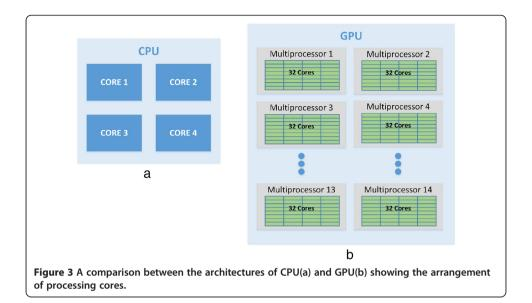
1000Tflops of processing power. This massive parallelism in GPU makes it a more appealing option for parallel computing applications.
