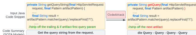
Figure 1: CodeAttack makes a small modification to the input code snippet (red) which causes significant changes to the code summary obtained from the SOTA pre-trained programming language models. Keywords are highlighted in blue and comments in green.
